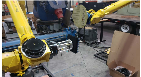
Fig. 9. Photograph of the dual 6-axis industrial robotic antenna measurement system undergoing preliminary factory testing.
